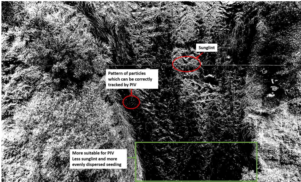
Figure 28: The figure shows the sunglints, that cause problems for the PIV analysis, along with correct seeding pattern that should be tracked.
