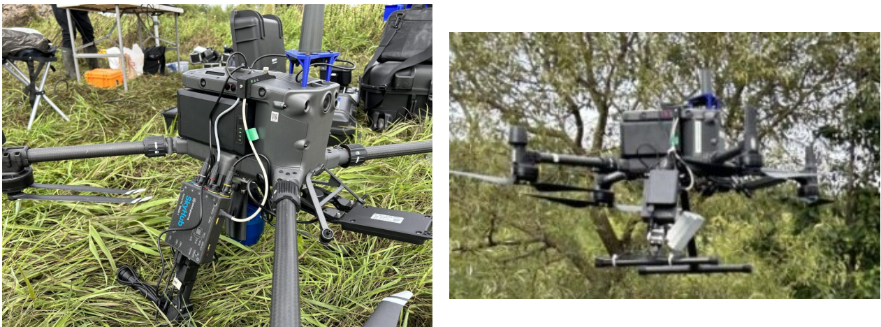
Figure 3: Left: The DJI Matrice 300 up close with the Skyhub onboard computer. Right: Doppler radar payload in flight, the radar is the white square mounted below the main body of the drone.
