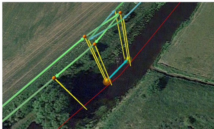
Figure 11 - 15m overlap between flight routes
