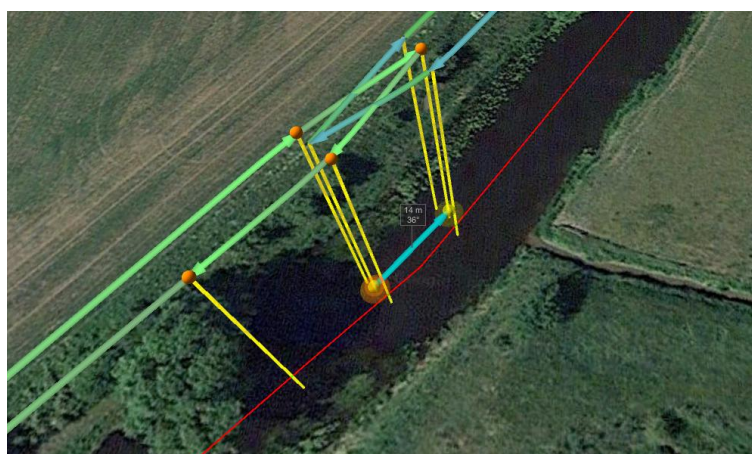
Figure 12 - 15m overlap between flight routes
