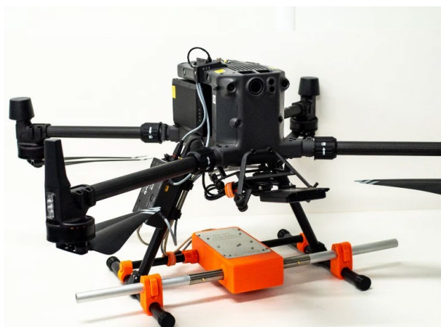
Figure 5 - DJI M300 RTK with Radar Systems Zond AERO LF GPR
