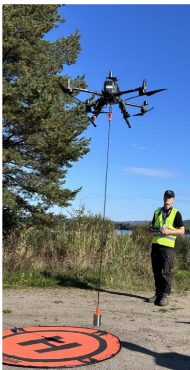
Figure 23 – Sonar Payload attached to DJI M300 RTK
