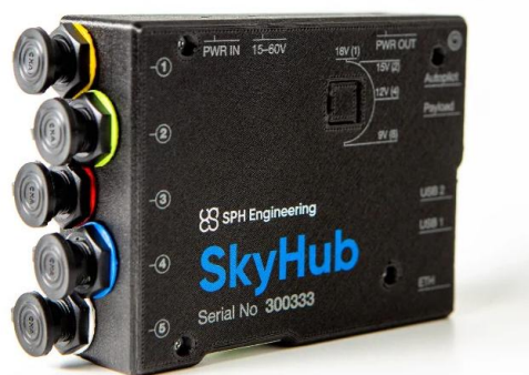
Figure 3 - SkyHub payload controller
