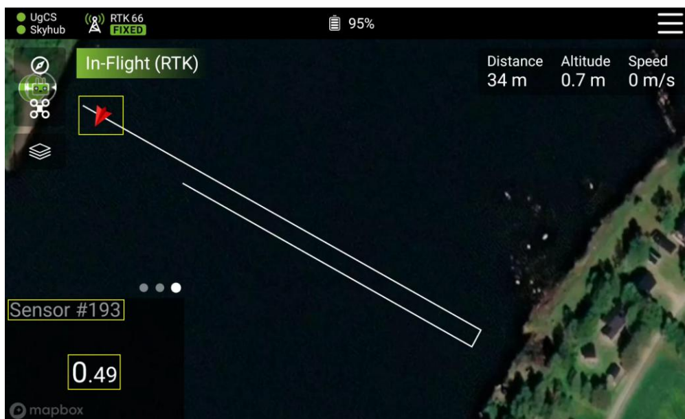
Figure 11 – Remote Controller View: Doppler radar payload in flight along the main flight line. Output in lower left corner reports surface velocity value. Barometric altitude in upper right corner is not in effect due to TFF mode.
