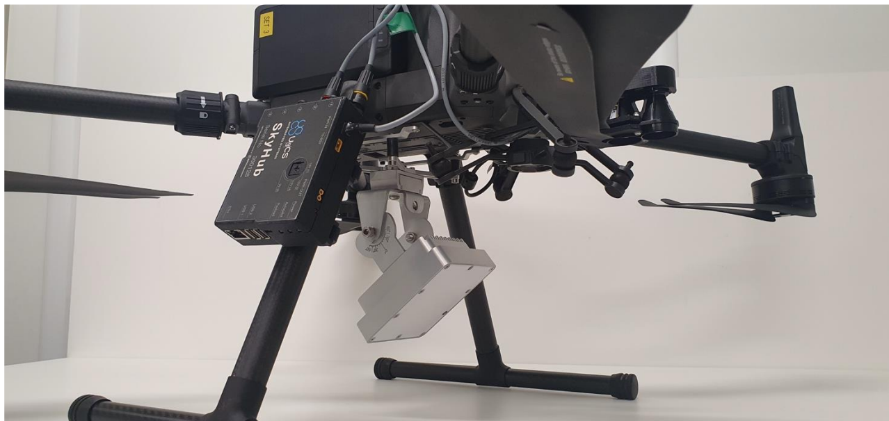
Figure 5 - DJI M300 RTK with Geolux RSS-2-300W Doppler Radar
